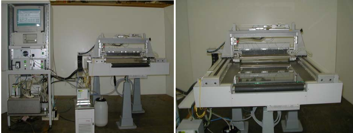
Figure 23: The programmable coating machine comprising the coating table, the control tower and the associated process equipment.
