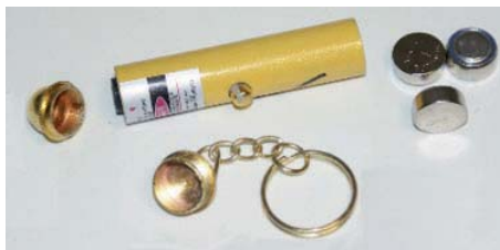
5 Disassembly of economical laser pointer
