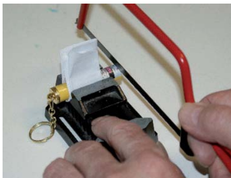
6 Cutting the collimating lens off laser pointer
